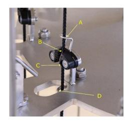
Force the spring-loaded bottom drawer "A" toward "B" at the centre of the sampler; the back side of "A" has an eye to be aligned beneath "B"  $^{\prime\prime}$
